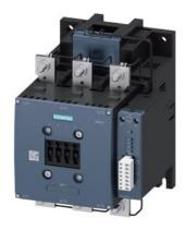
power contactor AC-1 500 A / 690 V / 40  $^{\circ}$ C 3-pole, Uc: 96-127 V AC(50-60 Hz) / DC PLC input 24 V DC drive: electronic auxiliary contacts 2 NO + 2 NC main circuit: busbar control and auxiliary circuit: screw terminal with remaining lifetime indicator
