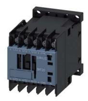
power contactor, AC-3e/AC-3, 9 A, 4 kW / 400 V, 3-pole, 220 V AC, 50 Hz / 240 V, 60 Hz, auxiliary contacts: 1 NC, ring cable lug connection, size: S00
