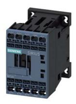
power contactor, AC-3e/AC-3, 12 A, 5.5 kW / 400 V, 3-pole, 24 V DC, 0.7-1.25\* Us, with integrated suppressor diode, auxiliary contacts: 1 NO, spring-loaded terminal, size: S00, suitable for PLC outputs, not expandable with auxiliary switch , upright mounting position
