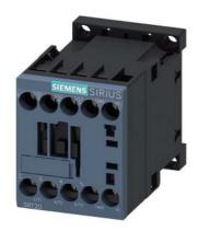
power contactor, AC-3e/AC-3, 16 A, 7.5 kW / 400 V, 3-pole, 230 V AC, 50/60 Hz, auxiliary contacts: 1 NO, screw terminal, size: S00, suspended mounting position
