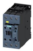
power contactor, AC-3e/AC-3, 41 A, 18.5 kW / 400 V, 3-pole, 21-33 V AC/DC, 50/60 Hz, with integrated varistor, auxiliary contacts: 1 NC, screw terminal, size: S2, F-PLC-IN
