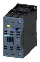
power contactor, AC-3e/AC-3, 41 A, 18.5 kW / 400 V, 3-pole, 175-280 V AC/DC, 50/60 Hz, with integrated varistor, auxiliary contacts: 1 NC, main circuit: screw terminal, control and auxiliary circuit: spring-loaded terminal, size: S2, F-PLC-IN
