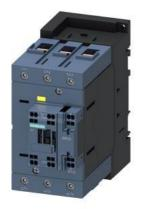
power contactor, AC-3e/AC-3, 95 A, 45 kW / 400 V, 3-pole, 83-150 V AC/DC, 50/60 Hz, with integrated varistor, auxiliary contacts: 1 NC, main circuit: screw terminal, control and auxiliary circuit: spring-loaded terminal, size: S3, F-PLC-IN
