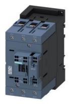
power contactor, AC-3e/AC-3, 110 A, 55 kW / 400 V, 3-pole, 230 V AC, 50/60 Hz, auxiliary contacts: 1 NO + 1 NC, main circuit: screw terminal, control and auxiliary circuit: spring-loaded terminal, size: S3
