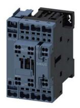
contactor AC-1, 35 A, 400 V / 40 °C, 4-pole, 24 V AC, 50 Hz, auxiliary contacts: 1 NO + 1 NC, spring-loaded terminal, size: S0, upright mounting position
