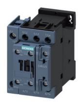
power contactor, AC-3, 32 A, 15 kW / 400 V, 4-pole, 48 V AC, 50/60 Hz, auxiliary contacts: 1 NO + 1 NC, screw terminal, size: S0  $\,$
