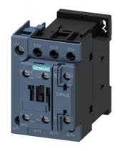
power contactor, AC-3, 32 A, 15 kW / 400 V, 4-pole, 230 V AC, 50/60 Hz, auxiliary contacts: 1 NO + 1 NC, screw terminal, size: S0  $\,$
