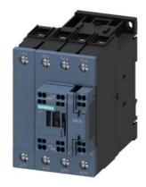
contactor AC-1, 110 A, 400 V / 40 °C, 4-pole, 20-33 V AC/DC, 50/60 Hz, with integrated varistor, auxiliary contacts: 1 NO + 1 NC, main circuit: screw terminal, auxiliary and control circuit: spring-loaded terminal, size: S2,
