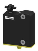
RFID safety switch with tumbler, plastic, open-circuit principle, actuator monitoring, 24 V DC, with auxiliary release, IP69, locking force 1150 N, individually coded multiple teach-in, coding level high according to ISO 14119, diagnostic output, M12 plug 8-pole, 3 LEDs for display of the operating states, 3 directions of actuation, latching force with turnstile adjustable: 25 N or 50 N. hygienic design. actuator 3SE6410-1AC01 to be ordered separately.
