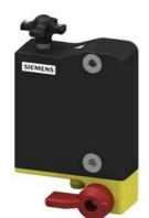
RFID safety switch with tumbler, plastic, with escape release, red levers can be mounted on both sides, quiescent current principle, tumbler monitoring, 24 V DC, IP69, locking force 1150 N, family-coded, diagnostic output, M12 plug 8-pole, 3 LEDs for display of the operating states, 3 directions of actuation, latching force with turnstile adjustable: 25 N or 50 N. hygienic design. actuator 3SE6410-1AC01 to be ordered separately.
