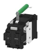
Contactor, Size 2, 2-pole, for railway applications DC-3 and 5, 7.5 A at 750 V 48V DC Auxiliary contacts 21 (2NO+1NC) with varistor and series resistor Operating range 0.7...1.25xUS
