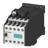
Contactor relay, 100E, EN 50011, 7 NO + 3 NC, screw terminal DC operation 33 V DC Integrated varistor
