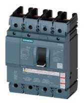
molded case switch 3VA5 UL frame 250 max short-circuit curr. rating 65kA @ 480 V 4-pole MCS110, In=150A without overload protection SELF PROTECTION Ii=16 x In w/o connection
