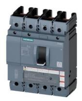
circuit breaker 3VA5 UL frame 250 breaking capacity class C 100kA @ 480 V 4-pole, line protection TM230, FTAM, In=225A overload protection Ir=225A fixed short circuit protection li=5...10 x In neutral protection 1 w/o connection
