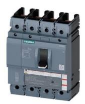
circuit breaker 3VA5 UL frame 250 breaking capacity class M 35kA @ 480 V 4-pole, line protection TM230, FTAM, In=90A without overload protection Ir=90A fixed short circuit protection Ii=5...10 x In neutral protection 1 w/o connection
