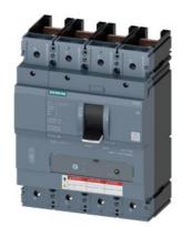
circuit breaker 3VA5 UL frame 400 breaking capacity class C 100kA @ 480 V 4-pole, line protection TM230, FTAM, In=200A overload protection Ir=200A fixed short circuit protection li=5...10 x In neutral protection 1 w/o connection
