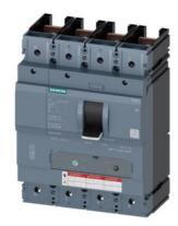
circuit breaker 3VA5 UL frame 400 breaking capacity class C 100kA @ 480 V 4-pole, line protection TM230, FTAM, ln=350A overload protection lr=350A fixed short circuit protection li=5...10 x In neutral protection 1 w/o connection
