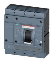
circuit breaker 3VA5 UL frame 800 breaking capacity class M 35kA @ 480 V 4-pole, line protection TM230, FTAM, In=600A overload protection Ir=600A fixed short circuit protection Ii=5...10 x In neutral protection 1 Al-lug, line and load side
