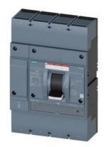
circuit breaker 3VA5 UL frame 800 breaking capacity class C 100kA @ 480 V 4-pole, line protection TM230, FTAM, In=700A overload protection Ir=700A fixed short circuit protection Ii=5...10 x In neutral protection 1 Al-lug, line and load side
