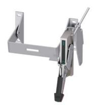
Operating Unit with Rod Variable Depth Flange Mounted operator kit, consisting of: handle steel chrome plated NEMA 4/4X black=OFF, red=ON Switching mechanism Mounting depth 8" to 16" Accessory for: 3VA5 400, 3VA5 600 3VA6 400, 3VA6 600
