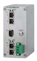
SIPLUS CMS-Hardware RPN "IEEE 1394B T002; IEEE 1394B" "Multi-port repeater; 2 opt." "and 1 electr. interface;" UW=24 V DC
