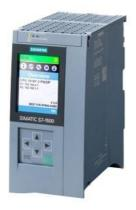
SIPLUS S7-1500 CPU 1516F-3 PN/DP based on 6ES7516-3FN02-0AB0 with conformal coating, -40...+60 °C, central processing unit with work memory 1.5 MB for program and 5 MB for data, 1st interface: PROFINET IRT with 2-port switch, 2nd interface: PROFINET RT, 3rd interface: PROFIBUS, 10 ns bit performance, SIMATIC Memory Card required
