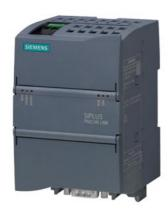
SIPLUS PN/CAN link based on 6BK1620-0AA00-0AA0 with conformal coating, -40...+70 °C, from PROFINET to CAN/CANopen networks CAN 2.0 A/B CANopen manager to CiA301/302 CANopen slave to CiA301/302 IP20
