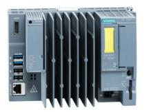
SIMATIC ET 200SP Open Controller, CPU 1515SP PC2 TF, 8 GB RAM, 128 GB CFast with Windows 10 IoT Enterprise 64-bit and S7-1500 Failsafe Software Controller CPU 1505SP TF pre-installed, Interfaces: 1x Slot CFast, 1x slot SD/MMC, 1x connection for ET 200SP bus Adapter PROFINET, 1x 10/100/1000 Mbit/s Ethernet, 2x USB 3.0, 2x USB 2.0, 1x display port, Documentation on CFast Restore image on CFast
