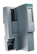
SIPLUS ET 200SP IM155-6PN ST TX rail based on 6ES7155-6AU01-0BN0 with conformal coating, -40...+70 °C, OT4 with ST1/2 (+85 °C for 10 minutes), PROFINET interface module, 1 slot for BusAdapter, max. 32 I/O modules, and 16 ET 200AL modules, single hot swap, including server module (6AG1193-6PA00-7AA0)
