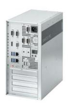
SIMATIC IPC527G (Box PC); Core i5-6500 (4C/4T, 3.2 (3.6) GHz); 1 TB HDD, internal; 8 GB DDR4; without operating system; 2x Gigabit Ethernet (IE/PN); 1x DisplayPort, 1x VGA; 4x USB 3.0, 2x USB 2.0; 2x RS232/485/422 (can be selected); 2x RS232, 1x 8 bit DIO, 2x PCI; 1x PCIe x16, 1x PCIe x1; 100/240 V AC power supply without line cable
