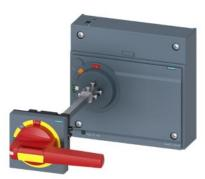
Door mounted rotary operator EMERGENCY-OFF NEMA type 1, 3R, 12, 4/4X with door interlocking, illumination kit 24 V DC and door open function accessory for: 3VA55/3VA65/3VA66
