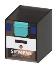
Plug-in relay, 4 changeover contacts 24 V DC, 6 A, Width 22.5 mm for LZS sockets
