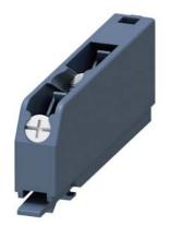
Removable terminal 2-pole, screw terminals up to maximal 2 x 1.5 mm2 or 1 x 2.5 mm2, For SIRIUS devices in industrial standard mounting rail enclosure
