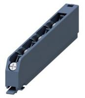
Removable terminal 4-pole, screw terminals up to maximal 2 x 1.5 mm2 or 1 x 2.5 mm2, For SIRIUS devices in industrial standard mounting rail enclosure
