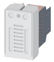
Accessory Circuit breaker 3WA, Arc chute, AC 1000 V frame size 1 only for fixed-mounted design height extension included in delivery package.
