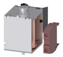
Accessory 3WA/3WL Shunt trip (ST) 5% OP, 208-240 V AC / 220-250 V DC momentary duty, with cut-off switch, not for continuous duty
