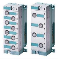
SIMATIC DP, Electronic modules for ET 200 PRO 4 DO 24 V DC, 2.0A High Feature, Channel diagnostics; short-circuit and wire break; incl. bus module, Connection module IO 6ES7194-4..00-0AA0 order separately
