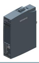
SIPLUS ET 200SP DI 16x24VDC ST TX rail based on 6ES7131-6BH01-0BA0 with conformal coating, -40...+70 °C, OT4 with ST1/2 (+85 °C for 10 minutes), digital input module, suitable for BU type A0, color code CC00, input type 3 (IEC 61131), sink input, (PNP, sinking input), input delay 0.05..20 ms module diagnostics for: wire break, supply voltage
