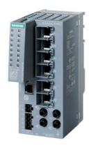
SIPLUS NET SCALANCE XC206-2 based on 6GK5206-2BB00-2AC2 with conformal coating, -40...+70 °C, manageable layer 2 IE switch; 6x 100 Mbps RJ45 ports; 2x 100 Mbps ST/BFOC ports; 1x console port; diagnostics LEDs redundant power supply temperature range -40 °C to +70 °C; assembly: DIN rail/S7 mounting rail/wall redundancy functions; office features (RSTP, VLAN,etc.); PROFINET IO device; Ethernet/IP-compliant C-Plug slot;
