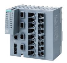
SIPLUS NET SCALANCE XC216-4C based on 6GK5216-4BS00-2AC2 with conformal coating, -40...+70 °C, manageable layer 2 IE switch; 12x 10/100 Mbps RJ45 ports; 4x 1000 Mbps combo ports (either 1000 Mbps SFPs or 10/100/1000 Mbps RJ45 ports can be used); 1x console port; diagnostics LEDs; redundant power supply temperature range -40 °C to +70 °C; assembly: standard mounting rail/S7 mounting rail/ wall; redundancy functions; office features(RSTP,VLAN,etc.); PROFINET IO device; Ethernet/
