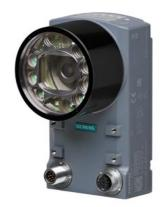
SIMATIC MV530 H optical reader Resolution: 1280 x 1024 pixels; Function: 1D/2D code reading; operating range [mm]: 30...250, depending on dot size; image field[mm]: 40x30...320x255; PoE; IP67; delivery: complete reader incl. built-in ring lamp green, pole filter, Optic 5.6 mm (fix- focus, fixed cover) and protective barrel;
