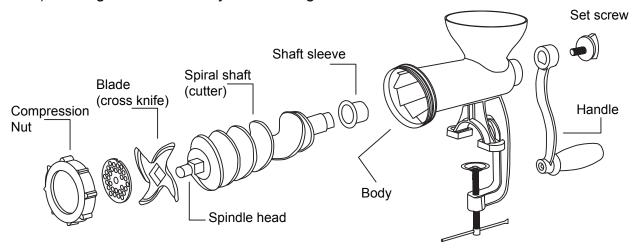
2) Making sausage: remove blade (3) and discharge plate (4), then install the plastic funnel (6) based on mincing meat structure.
