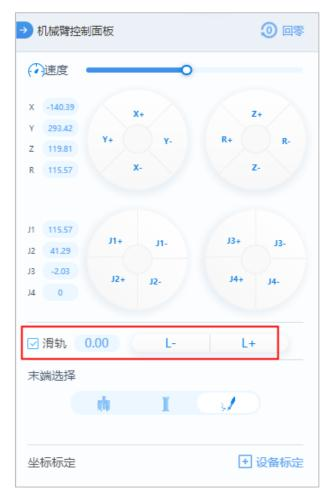
Figure 5.43 Enable sliding rail
