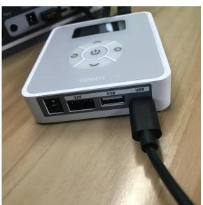
Figure 3.4 Connect Magician Lite to electrical outlet
