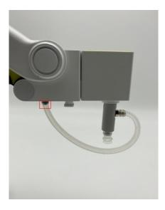
Figure 5.58 Install an air tube
