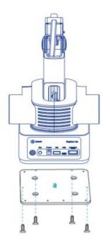
Figure 5.35 Fix plate a
