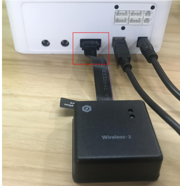
Figure 5.177 Connect with WIFI kit
