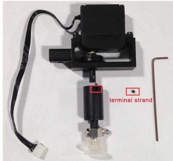
Figure 5.12 Dismantle the suction cup
