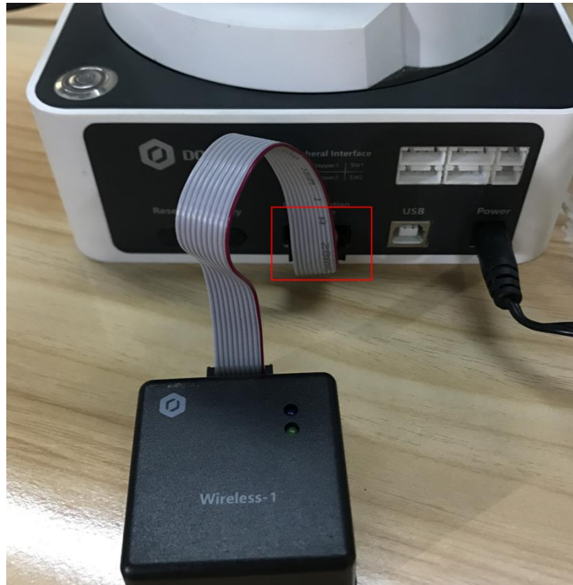
Figure 5.182 Connect with Bluetooth kit
