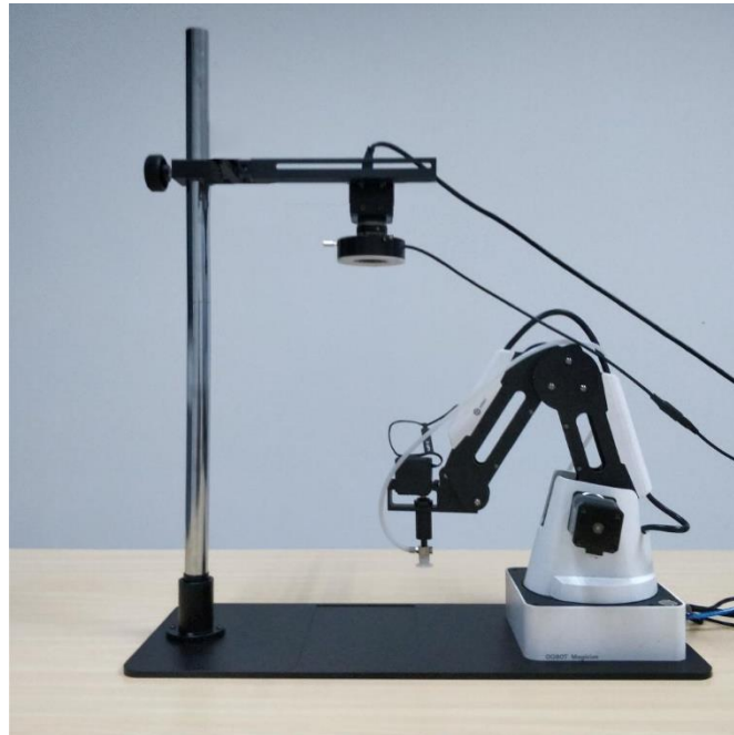
Figure 2.21 Install Dobot Magician
