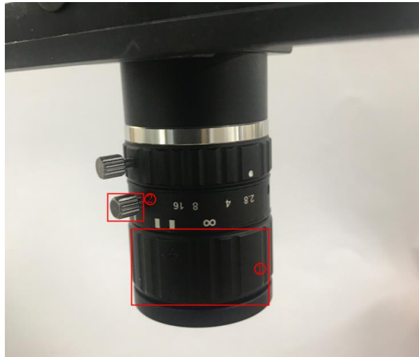
Figure 2.13 Adjust focal length
