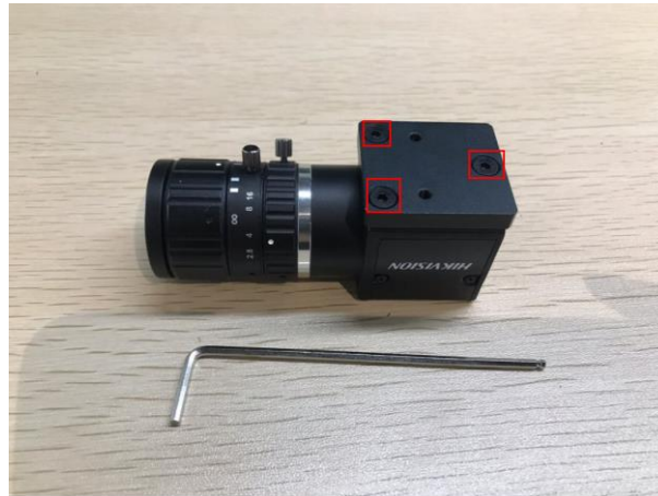
Figure 2.7 Fix camera plate
