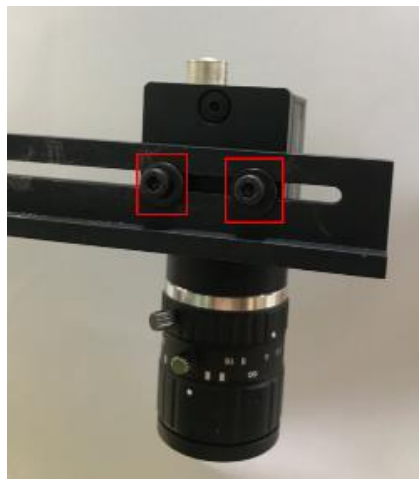
Figure 2.8 Fix camera mounting plate
