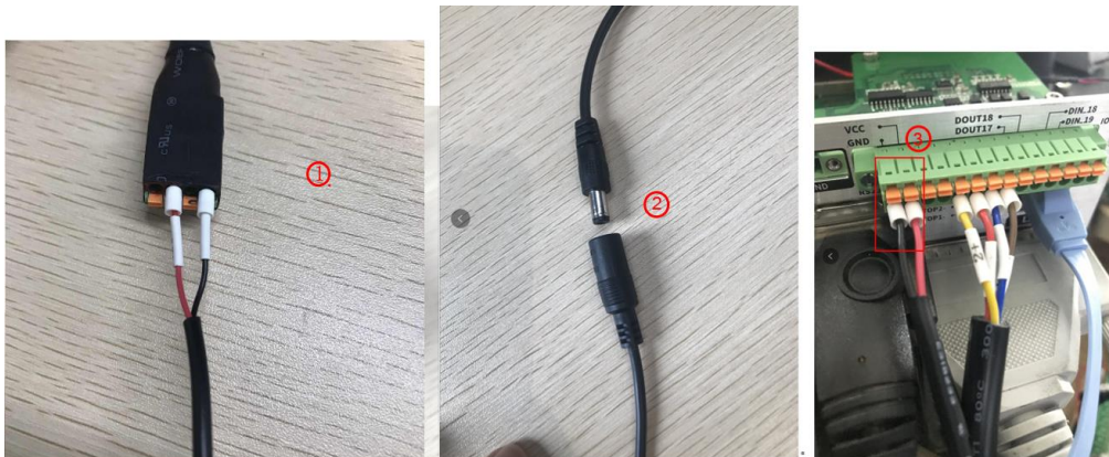
Figure 2.19 Connect light source switch
