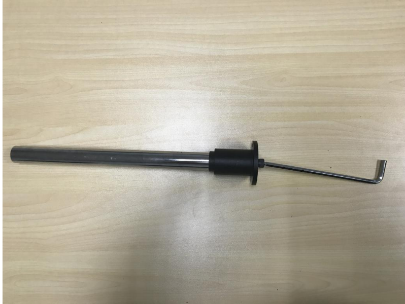
Figure 2.1 Install camera flange support
