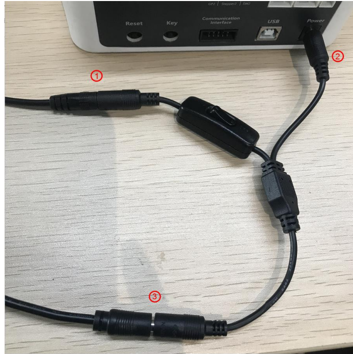
Figure 2.18 Connect light source switch
