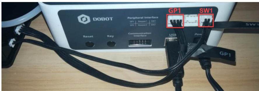
Figure 8.2 Air pump Connection
