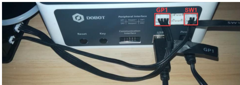
Figure 9.2 Air pump Connection
