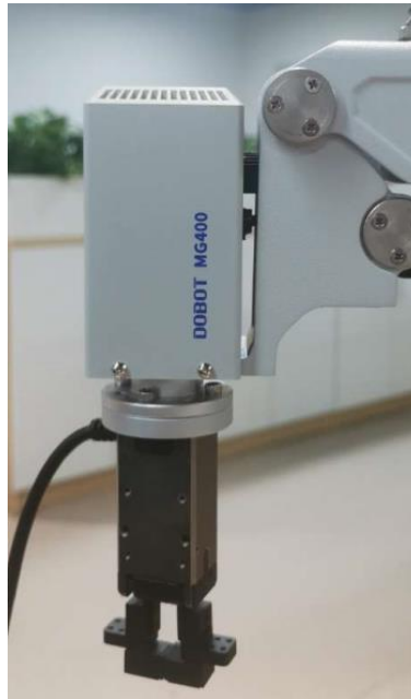
Figure 3.8 Install electromagnetic gripper
