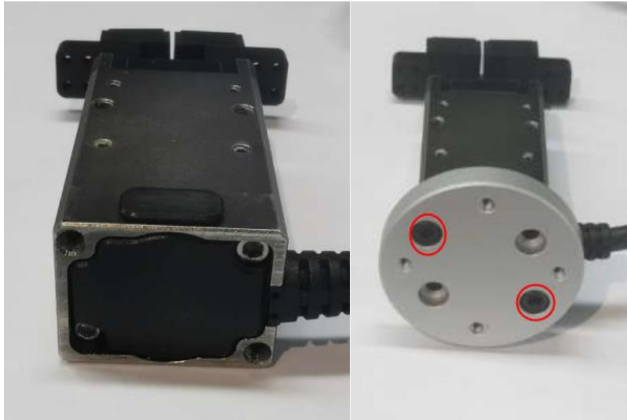
Figure 3.6 Install gripper mounting plate
