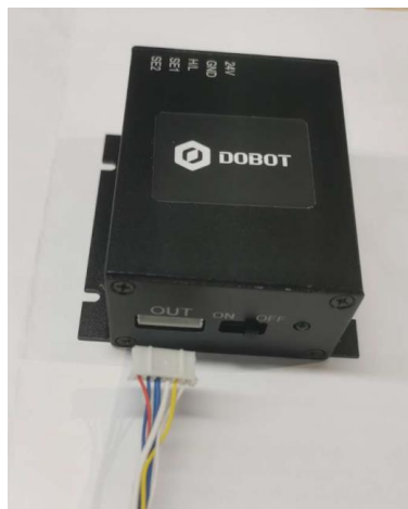
Figure 3.9 Connect electromagnetic gripper to control box
