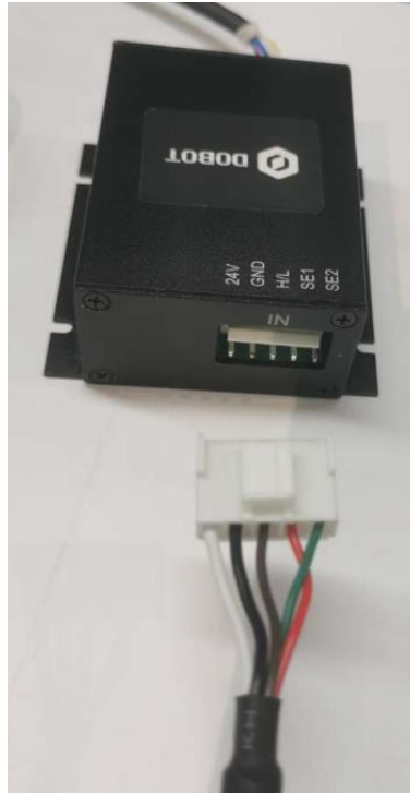
Figure 3.10 Connect gripper cable to control box
