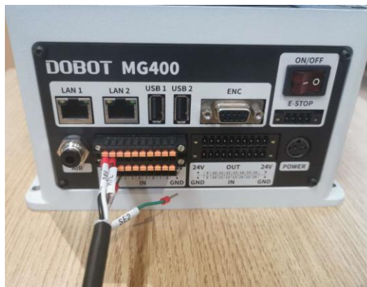
Figure 3.11 Connect gripper cable to MG400
