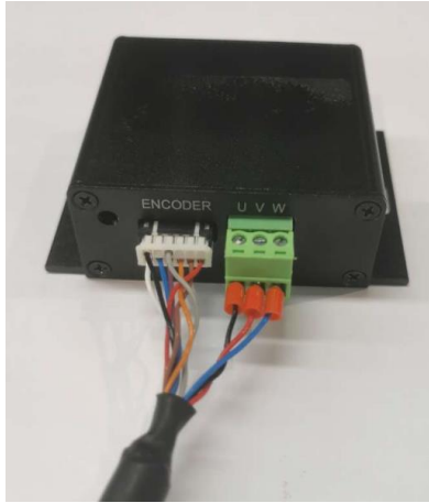
Figure 2.10 Connect servo gripper to controller
