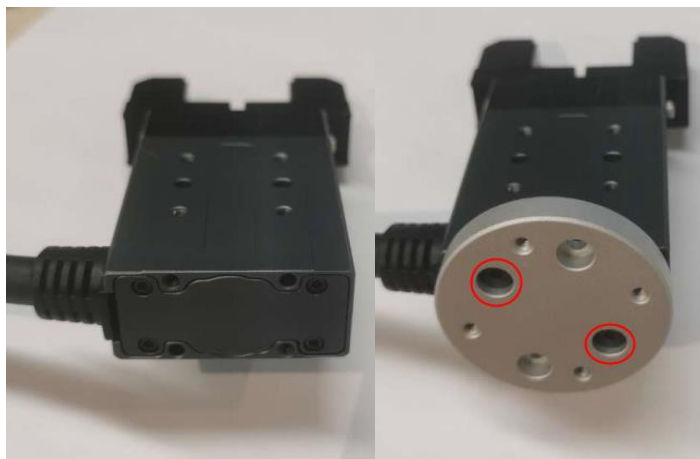
Figure 2.7 Install gripper mounting plate
