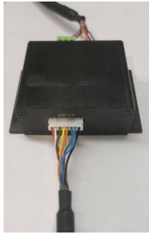
Figure 2.11 Connect gripper cable to controller
