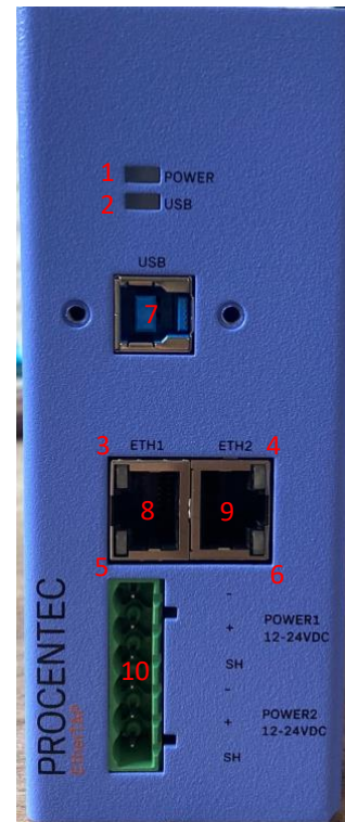
Figure 2: Identification of connections and LEDs for the 1Gbit/s version
