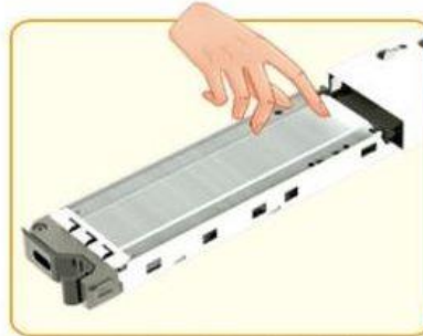
Press down the rear side till the latch is fastened, the installation is finished
